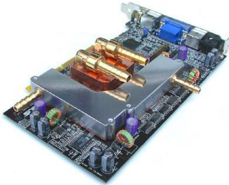
A watercooled graphic card. Handiwork by BladeRunner - Zero Fan Zone.
